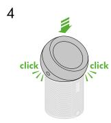
Firmly push the ball back into position, making sure it clicks securely into place.
